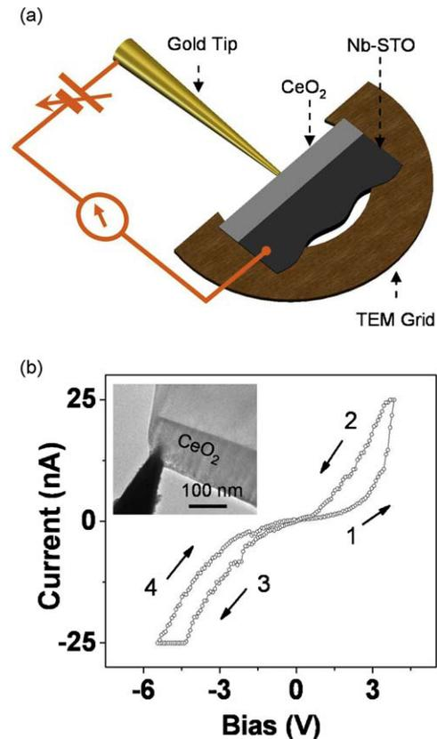
**Fig. 2.** (a) Scheme of *in situ* TEM measurement setup. The cross-section TEM-ready sample, CeO<sub>2</sub>/Nb-STO junction, was contacted by a gold tip at a selected position by piezo-controller, measuring the resistance and monitoring the structural evolution simultaneously. (b) A loop of *in situ* *I*–*V* sweep reveals the resistance switching effect. The inset: TEM image of metal-tip/CeO<sub>2</sub>/Nb-STO structure.
