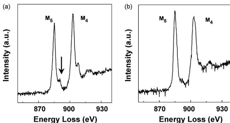
**Fig. 4.** (a) EEL spectra of Ce-M edge at zero bias. (b) A reversal in the intensity of Ce M<sub>45</sub> white lines was observed; and the shoulder indicated by arrow in (a) disappeared after applying the electric field.
