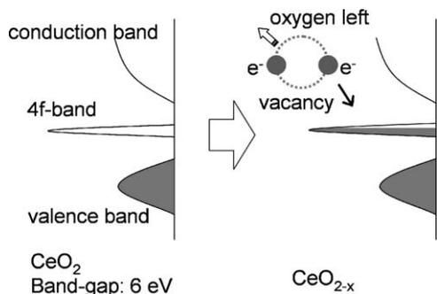
**Fig. 5.** Left: the energy band of perfect  $\text{CeO}_2$ , whose band gap is 6 eV (Koelling et al., 1983). There is a narrow empty Ce 4f band in the gap. Right: the energy band of  $\text{CeO}_{2-x}$ . When an oxygen atom moves away from their lattice positions, the two electrons will localize on cerium atoms (transition from  $\text{Ce}^{4+}$  to  $\text{Ce}^{3+}$ ). Thus, the electron conductivity is enhanced.
